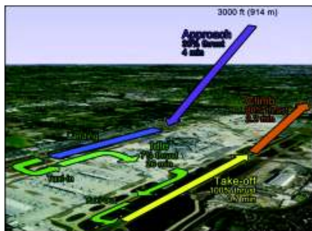
Fig. 5. Standard ICAO LTO cycle. Adapted from ICAO (2011).
